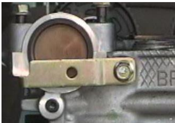
The CAS blanking plate bracket
